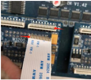
Correct(metal part to metal part)
